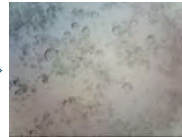
Viscous emulsion of coalesced droplets
